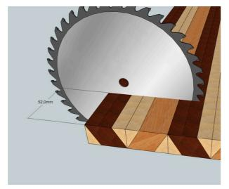
Set the table saw rip fence on the level of 52 mm.
