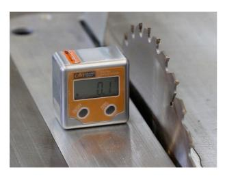
It is very important to set right angle of saw blade. Put the digital angle gauge at the table and press "ZERO".
