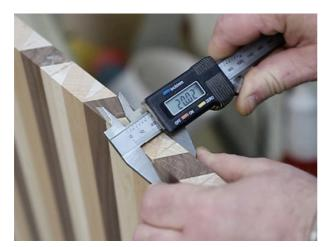
Check the thickness. Exactly 20 mm.
