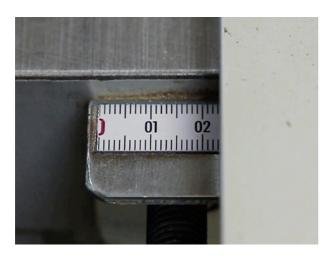
The final thickness of the walnut and beech panels must be 20 mm. So set the rip fence of the table saw on the level of 23 mm. 3 mm will be removed during planning. Usually 2 mm is enough. It is up to you.
