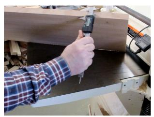
Check the 20 mm thickness. It is very important to be precise at this stage.
