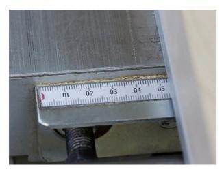
Set the rip fence of the table saw on the level of 53 mm.
