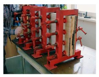
Clamp the boards. It is extremely important to compress well in the middle. I use specially made clamps that allow me to compress the board width of 400 mm. Do not make the boards wider than 200-300 mm using ordinary clamps.
