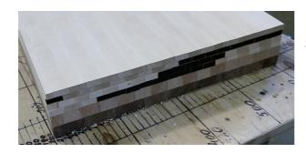
Make the width of all six panels the same for more convenient gluing.
