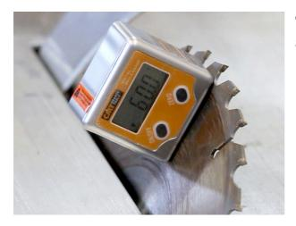
Tilt the saw blade and set the exact angle of 60 degrees.
