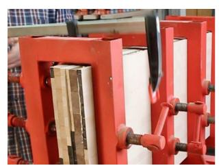
You can make 200-300 mm width board and use large F-clamps. They can clamp at the distance of 125 mm from the side of the board.
