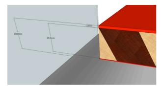
Plane the boards. You should remove 1,5 mm from each side.
