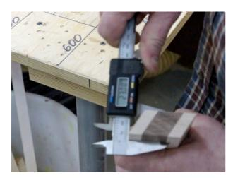
Check the thickness - 23 mm. The final thickness should be 20 mm. 3 mm will be removed later.
