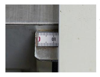
Then set the rip fence of the table saw on the level of 13 mm.
