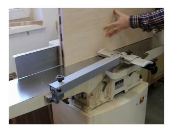
Align one edge of the boards on the jointer.
