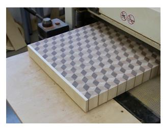
Sand the board. Cut off the edges, sand them, make finger slots and so on (not shown).
