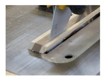
Cut off the corners. The cutting line must pass exactly at the corners of the internal rhombus.
