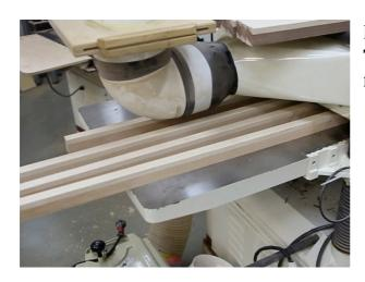
Plane the slats. Try to remove equal amount of material from both sides.
